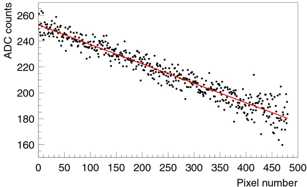
Capture of signal electrons by bulk defects causes Charge Transfer Inefficiency (CTI).
