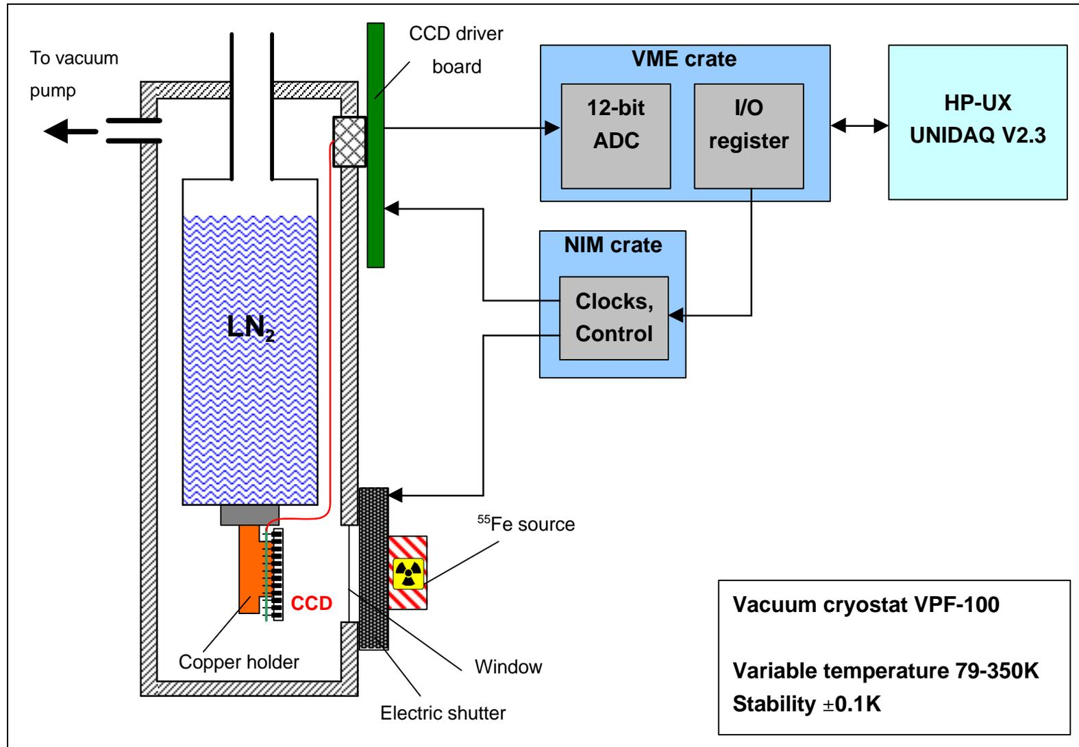
**Radiation Resistance of a Two-Phase CCD Sensor**
