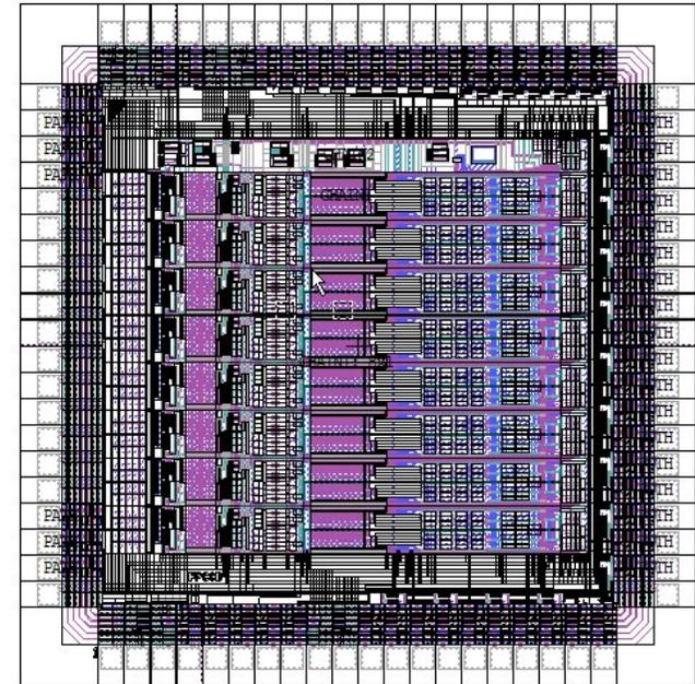
Readout ASIC with package
