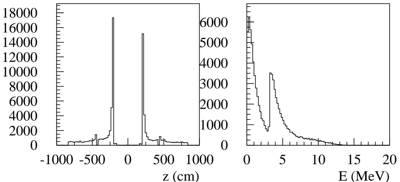
Neutron production point      Neutron kinetic energy
