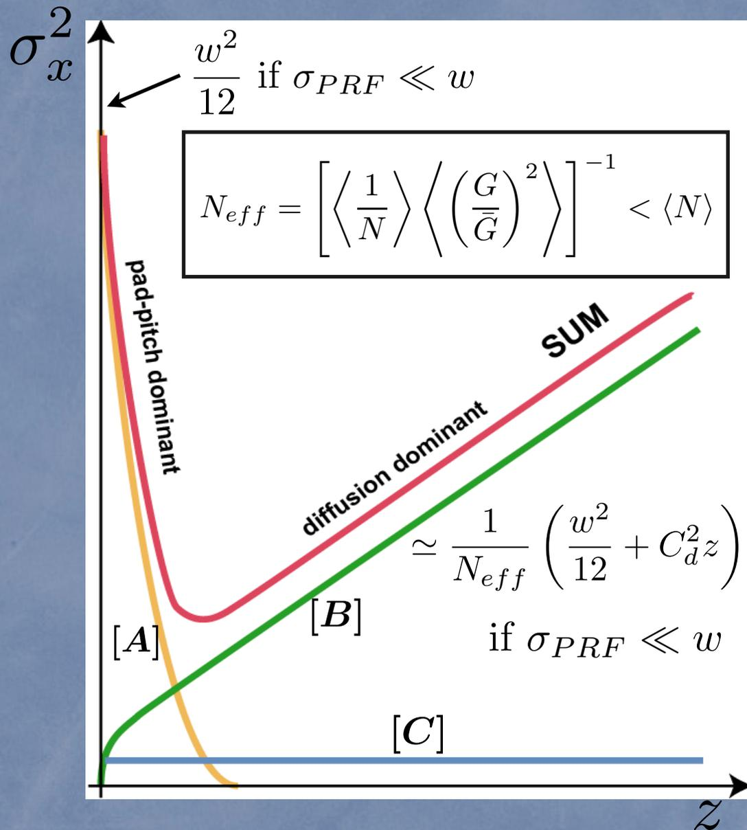
[A] Purely geometric term (S-shape systematics from finite pad pitch): rapidly disappears as  $Z$  increases
