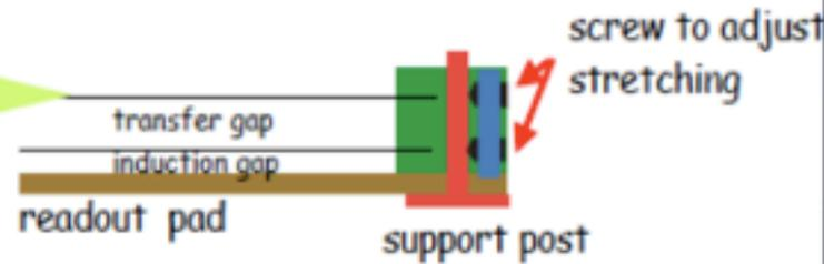
Transfer gap  $\sim 4\text{mm}$  : enlarge signal distribution (+2mm) width  $> 0.3 \times$  pad pitch
