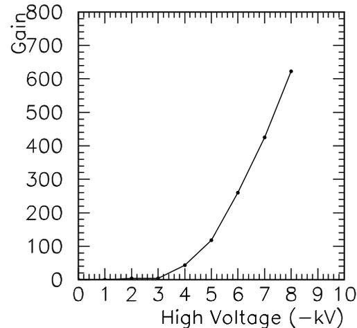
Gain vs. Photo-cathode voltage for proximity-focused EBCCD
