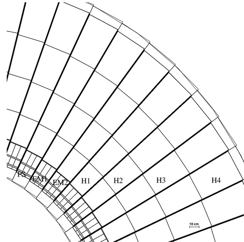
**Configuration of Baseline Barrel Calorimeter**
