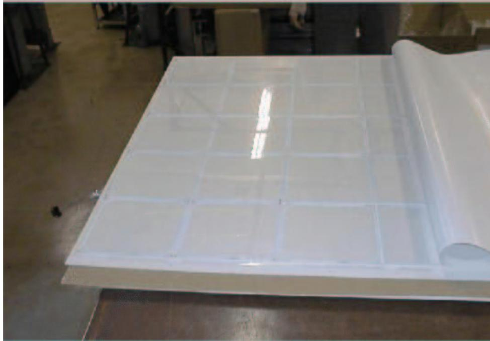
**Scintillator tiles arranged as  $5 \times 5$  segmentation**
