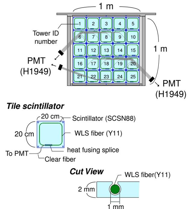
Schematic view of HCAL test module with Tile/Fiber configuration
