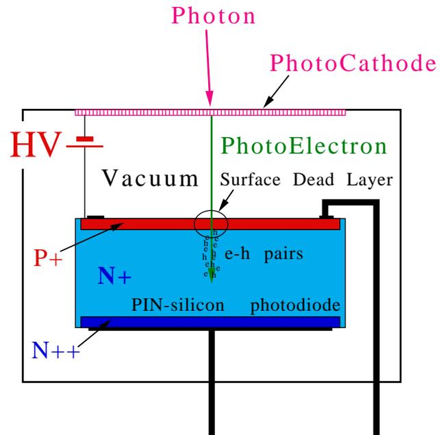
Schematic view of the HPD structure
