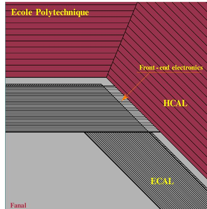
Barrel Calorimeter of TESLA
