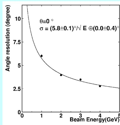
Angular resolution of shower axis measured by scintillator-strip-array EMcal.
