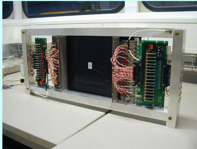
direct-mount ADP-readout scintillator-strip array
