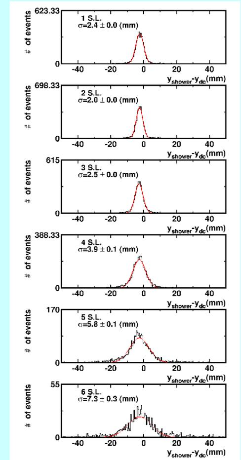
Position resolution for each super-layer of scintillator-strip-array EMcal.
