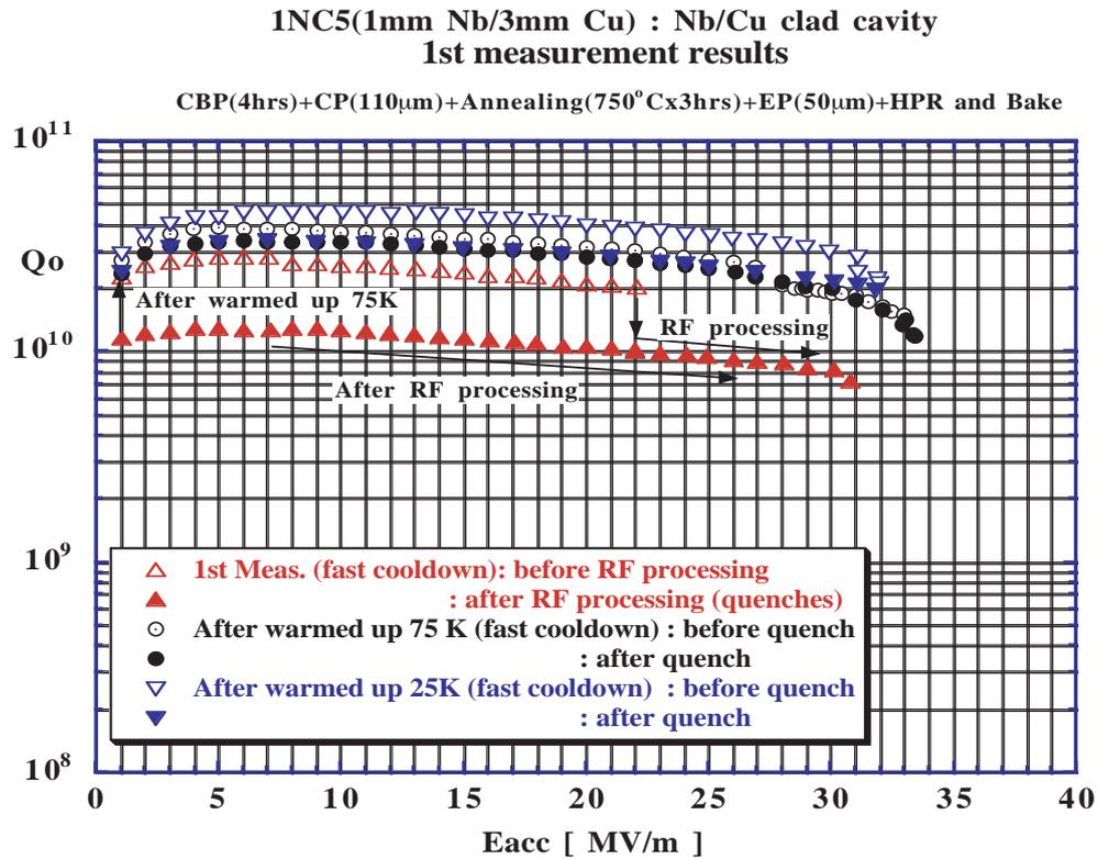
Figure 15: Recent result of Nb/Cu clad cavity in KEK/DESY.
