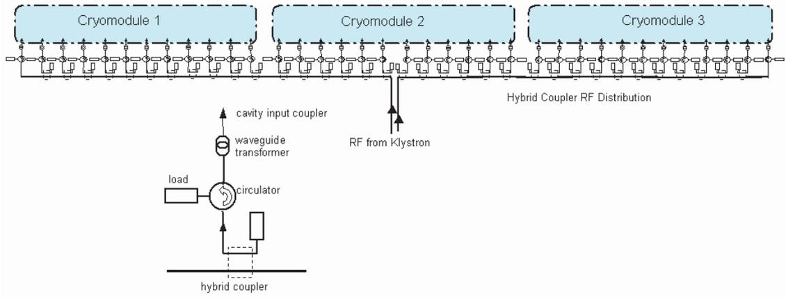
Figure 2: RF waveguide distribution of one RF station. Reproduced from Figure 3.3.5 in TDR II-97.
