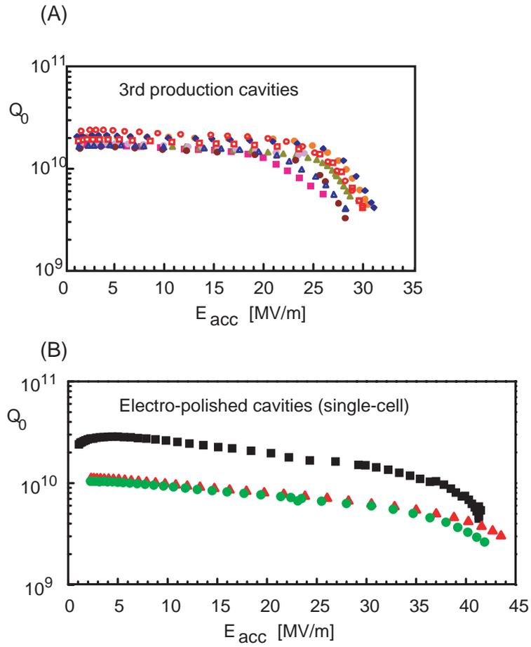
Figure 11:  $Q$  vs  $E_{acc}$  curves for: (A) 3rd production cavities (Image reproduced from Figure 2.1.10 in p.II-32 of TDR). (B) Electro-polished single-cell cavities (Reproduced from Figure 2.1.14 in p.II-37 of TDR)
