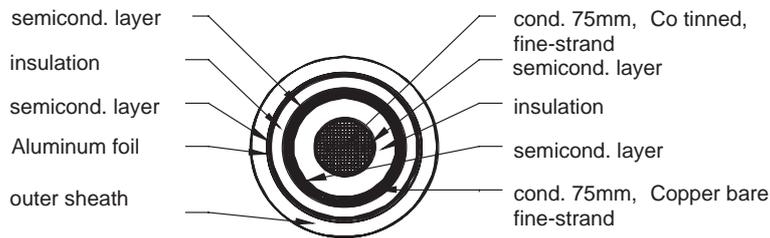
Figure 8: Construction of the pulse cable. Reproduced from Figure 3.3.4 of TDR II-93.
