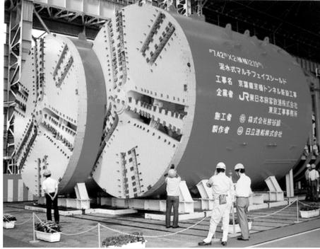
Figure 5: An example of a “dual-TBM” machine that was used for excavating a subway tunnel in the Tokyo area.
