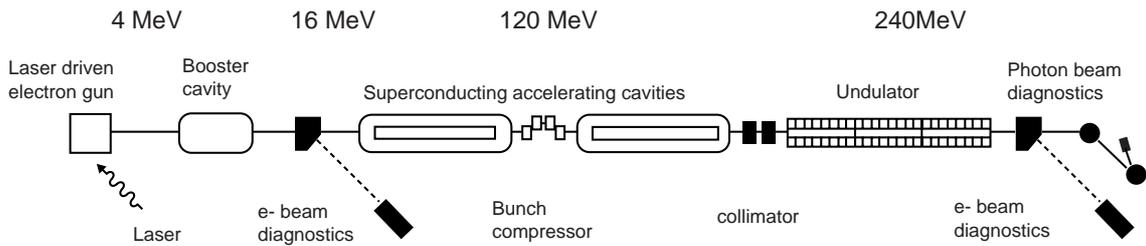
Figure 3: Schematic layout of TTF. Reproduced from Figure 2.2.1 in TDR II-49.
