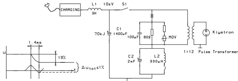
Figure 7: Conceptual circuit diagram of the TESLA modulator. Reproduced from Figure 3.3.3 of TDR II-91.
