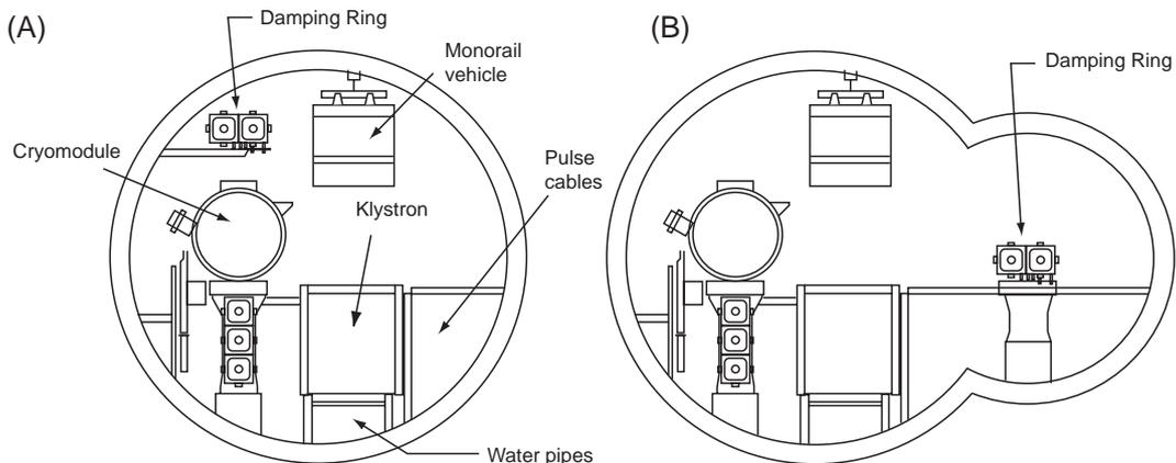
Figure 4: (A) Layout in the main linac tunnel that is explained in TESLA TDR (Image traced from Figure 8.2.7 in p.II-234). (B) Another possibility, drafted by a KEK delegate member. A TBM machine as shown in Fig. 5 might be applicable here.
