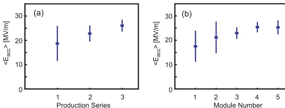
Figure 9: Average accelerating gradients at  $Q_0 > 10^{10}$ , measured in the vertical cryostat of : (a) the cavities in the three production series; and (b) the cavities installed in the first five cryomodules for TTF. (Reproduced from Figure 2.1.11 in p.33 of TDR)
