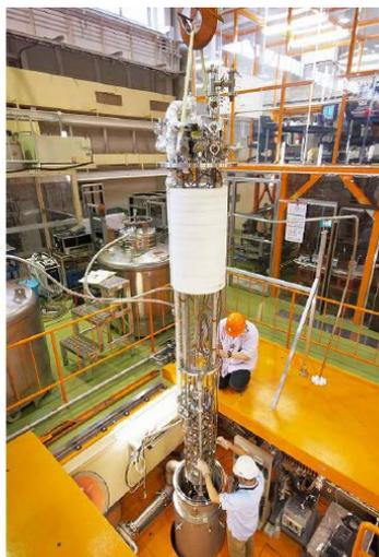
Vertical test of 9-cell cavity
