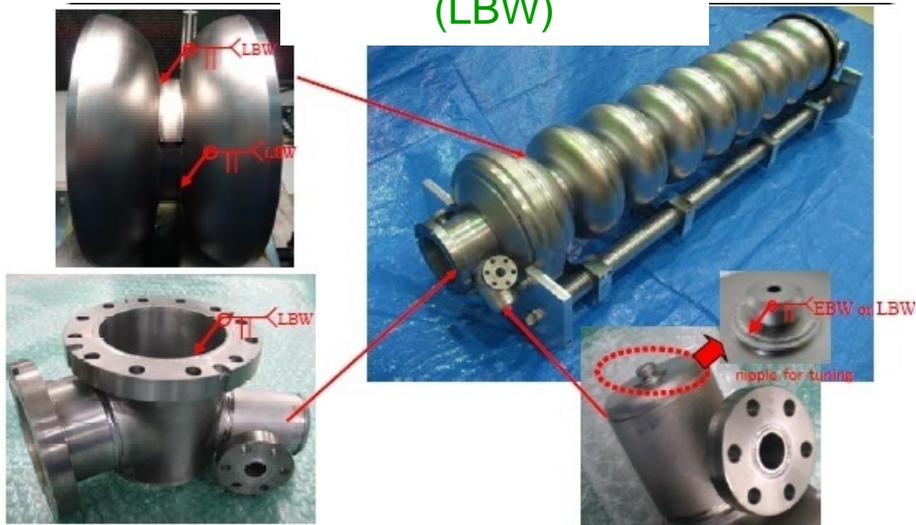
MHI-B 2-cell cavity (seamless dumbbell)
