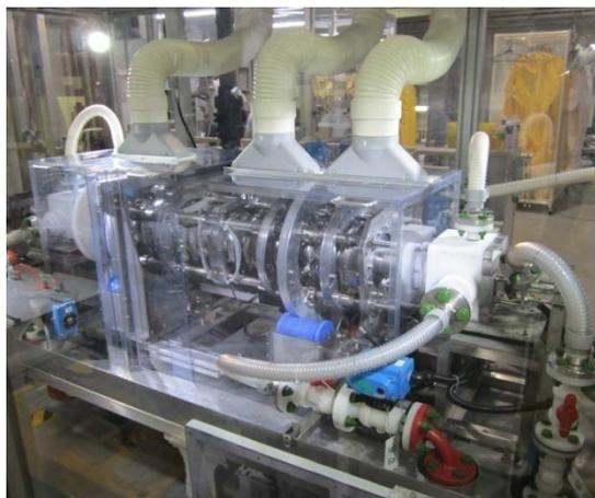
Electro polish (100μm removal)
