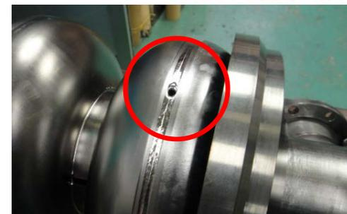
EBW failure (a hole at end-cell)
