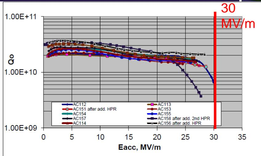
$Q_0(E_{acc})$  performance of the LG cavities AC112- AC114, AC151-AC158 at 2K after 50-120  $\mu\text{m}$  EP, 800° C, baking.
