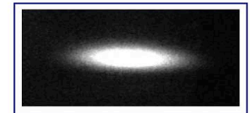
Beam image (x:46.2, y:10.2 μm)
