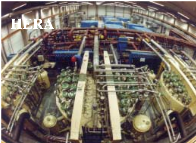
Fig. 6: Cryogenic system (consisting of 12 cryogenic units supplied from 7 refrigeration halls)
