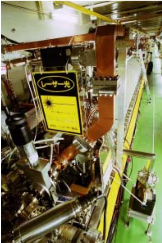
Figure 4: The RF gun implemented at ATF. Bronze wave guide to feed RF field to the gun is shown in the middle.
