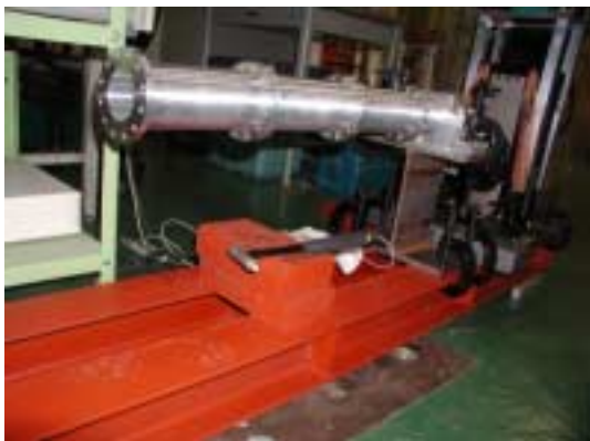
Figure 1: The 1/10 model of the support tube for the test of rigidity.
