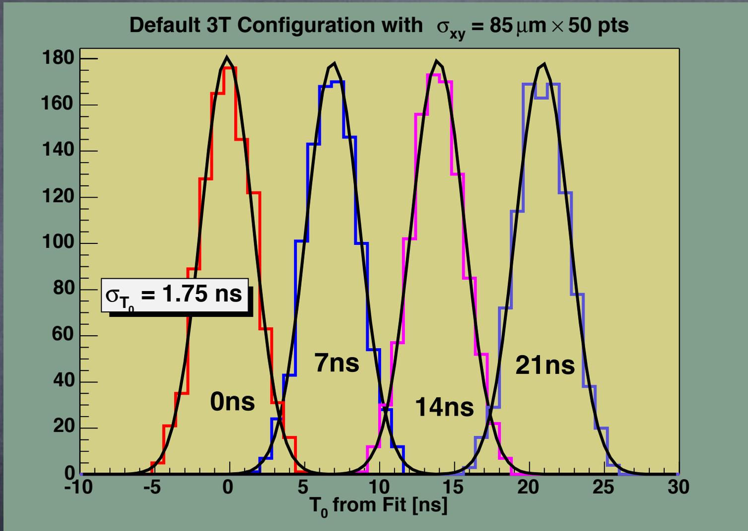
We can determine T0 with  $\sim 1.8 \text{ ns}$  accuracy as expected!
