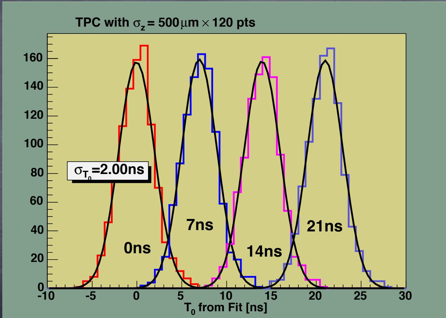
We can determine  $T_0$  with  $\sim 2.0\text{ns}$  accuracy as expected!
