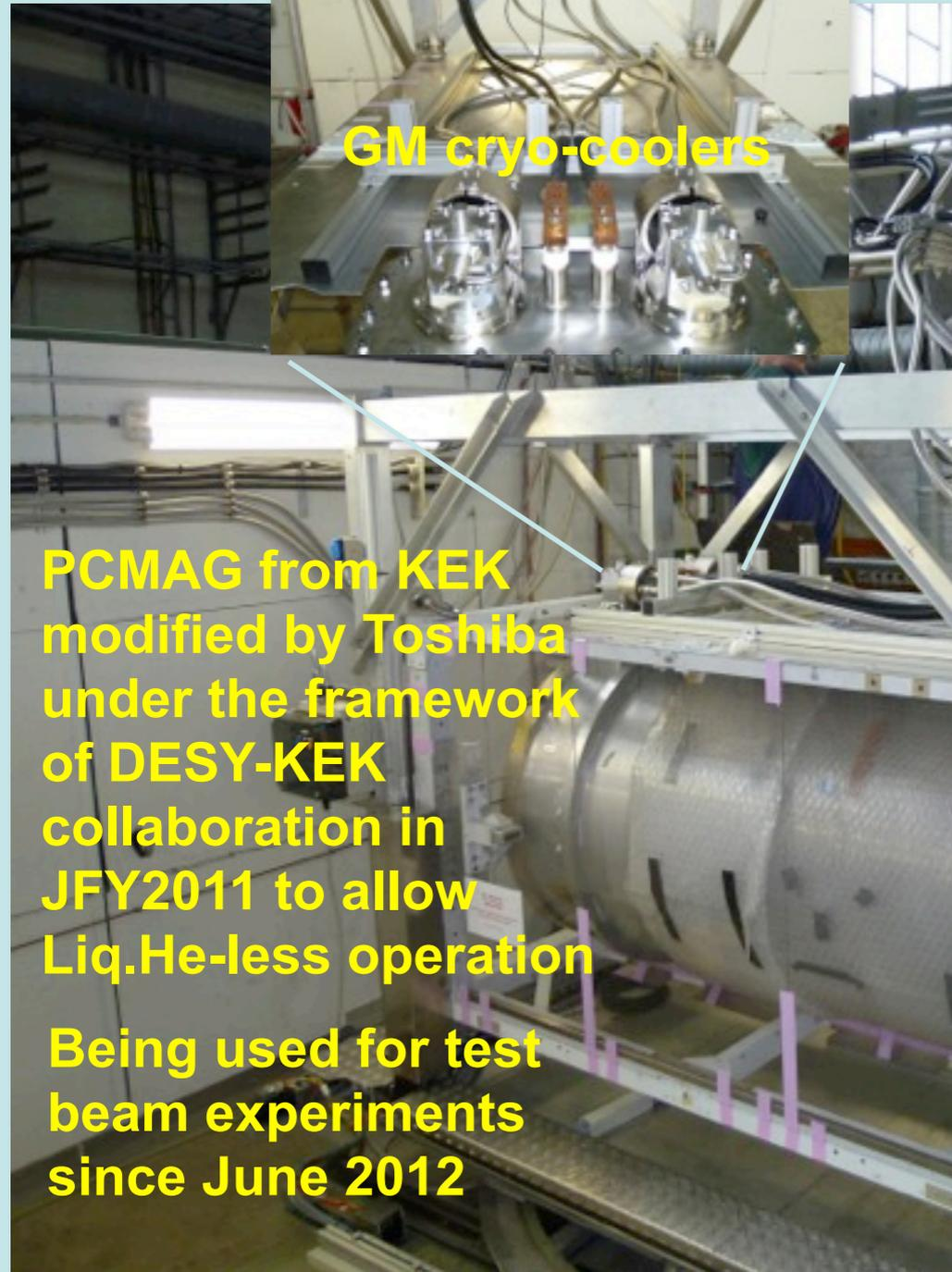
PCMAG from KEK modified by Toshiba under the framework of DESY-KEK collaboration in JFY2011 to allow Liq.He-less operation
