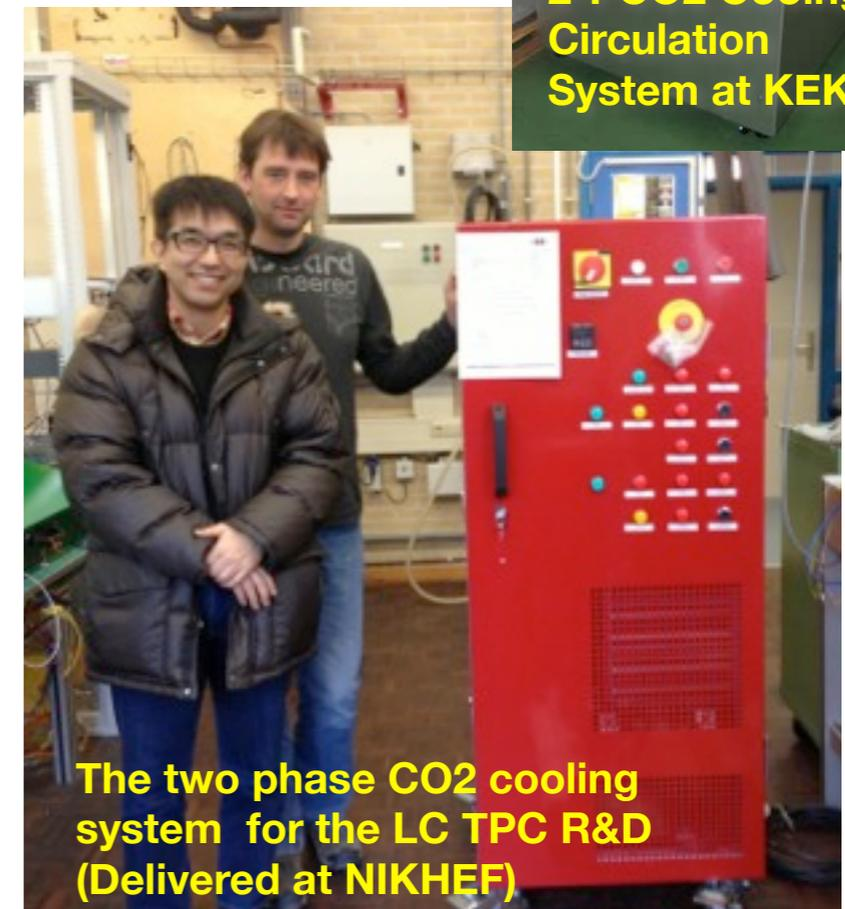
The two phase CO2 cooling system for the LC TPC R&D (Delivered at NIKHEF)
