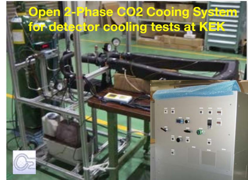
Open 2-Phase CO2 Cooling System for detector cooling tests at KEK
