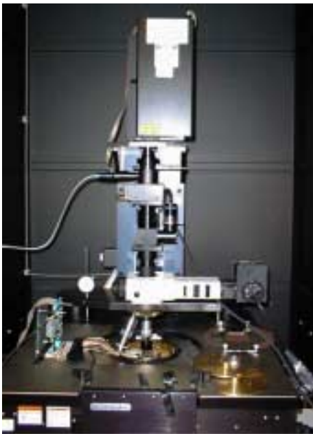
Figure 2: Laser scanner system for resolution study of CCDs.
