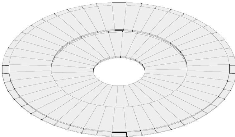
The sensor arrangement; the top side faces the IP.
