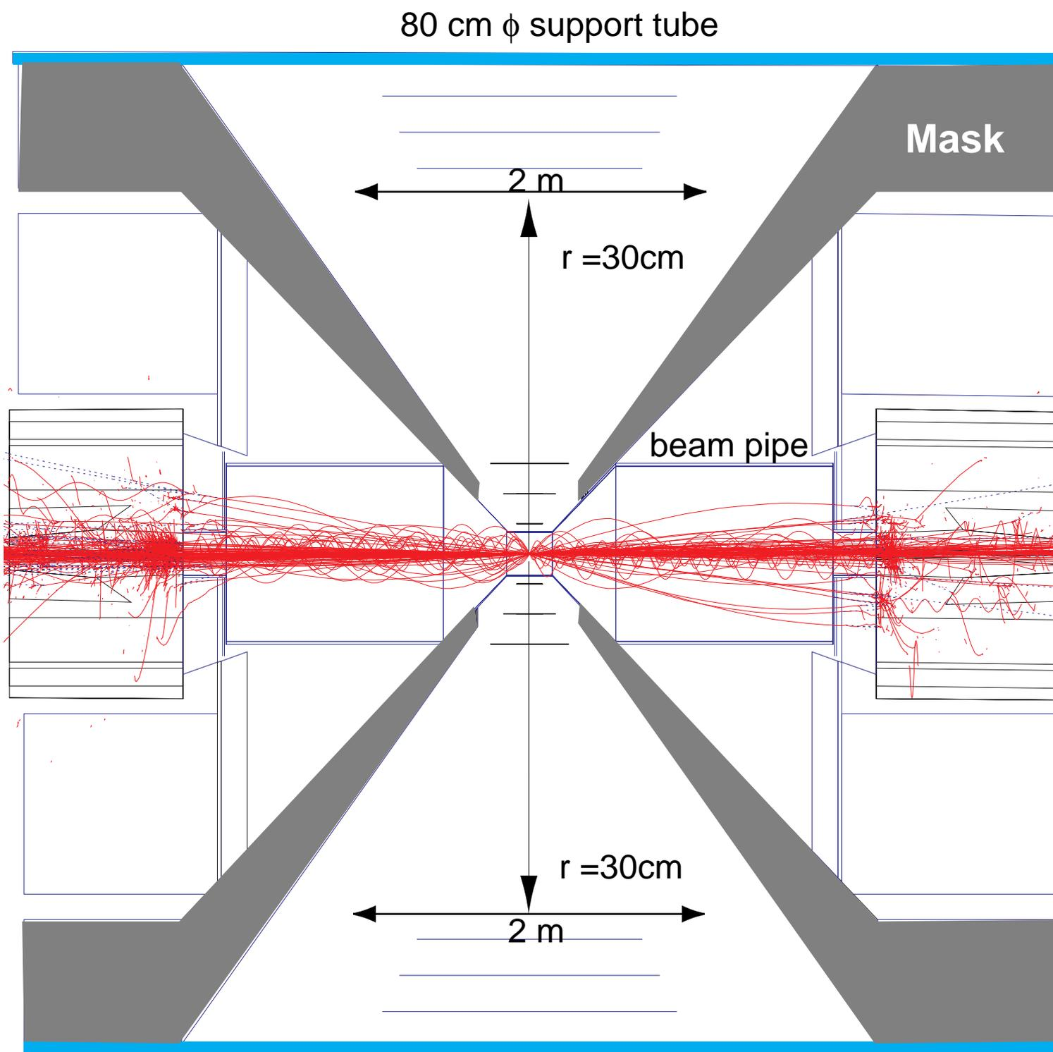
1/100 bunch and  $E_\gamma > 100\text{MeV}$ ,  $E_e > 10\text{MeV}$  for display purpose
