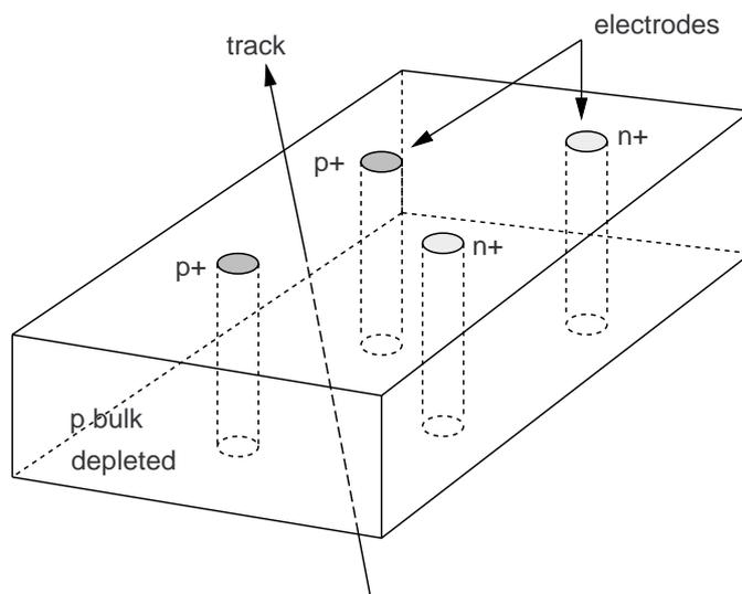
Schematic diagram of the 3D pixel concept
