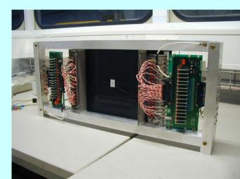
direct-mount ADP-readout scintillator-strip array
