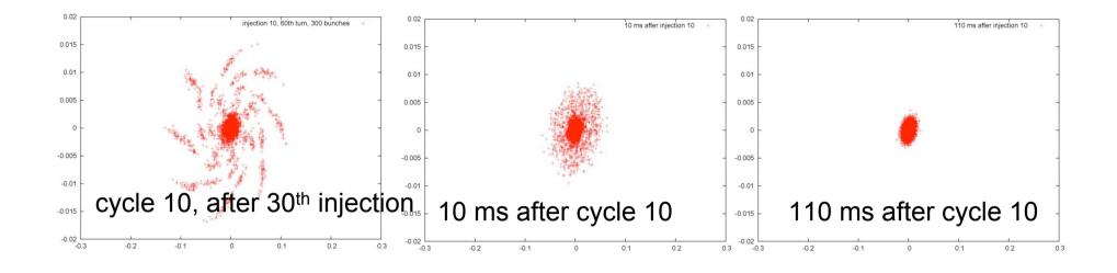
76% of injected e+ are lost! for a single cycle: 35% loss
