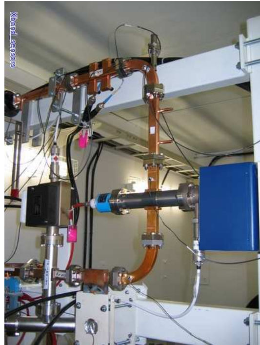
Figure 13: A waveguide of the X-band test stand equipped with acoustic sensors.
