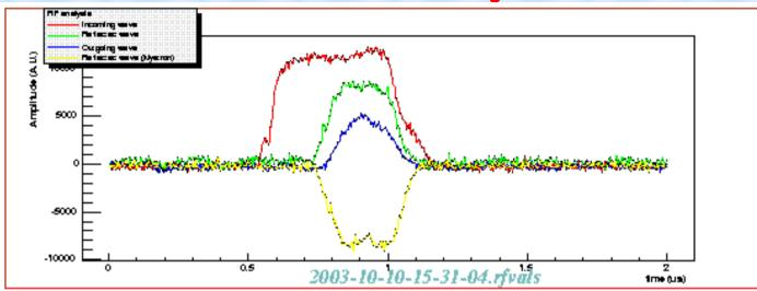
Difference between the end of the outgoing wave and the arrival of the reflected wave gives the position of the breakdown (t>0 = > bkdn close from input)
