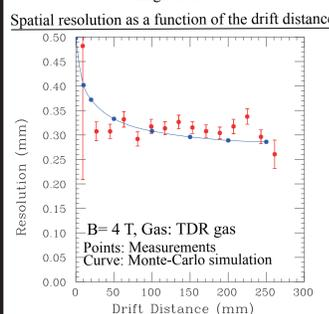
The measured spatial resolution as a function of the drift distance is compared to the Monte-Carlo simulation taking into account the ExB effect given by the Garfield simulation. It should be noted that the measured spatial resolution is almost constant over the measured range of drift distance. The simulation shows the improvement of resolution with increasing drift distance because of the de-clustering effect.
