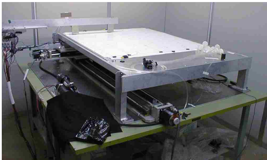
Figure 9.19: Automatic measurement stage for photo-electron yield uniformity.
