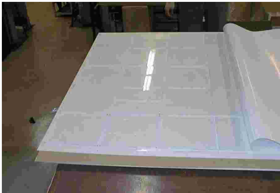
Figure 9.18: Scintillator tiles arranged as 5 \times 5 on the fiber-routing plate, and covered with white PET films.
